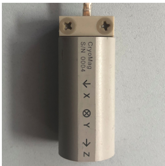
Figure 6: Axis orientations of the x, y and z axis on the three-axis sensor.
